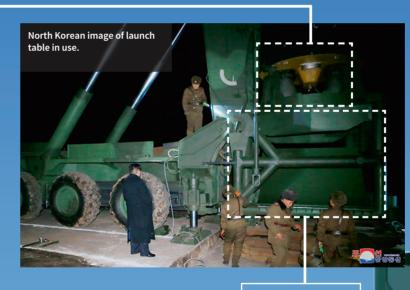
The use of a launch table has precedents in Soviet missile design. Examples of Soviet systems incorporating this design include the R-5/8A62 (SS-3 'Shyster') missile system, or the missile family of R-12/8K63 (SS-4 'Sandal'), R-14/8K65 (SS-5 'Skean'), and R-16/8K64 (SS-7 'Saddler'). However, this launch mode was phased out in the 1960s.
